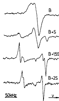
Figure 2. Variation of the 11 B NMR spectra in the system B-S as a function of composition.
